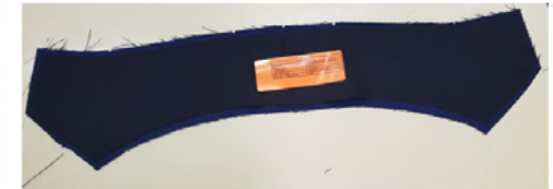
Fig: Collar cut using rotary
