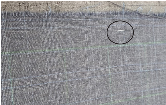
Fig: Use of staples on Ruizhou Machine Bed
