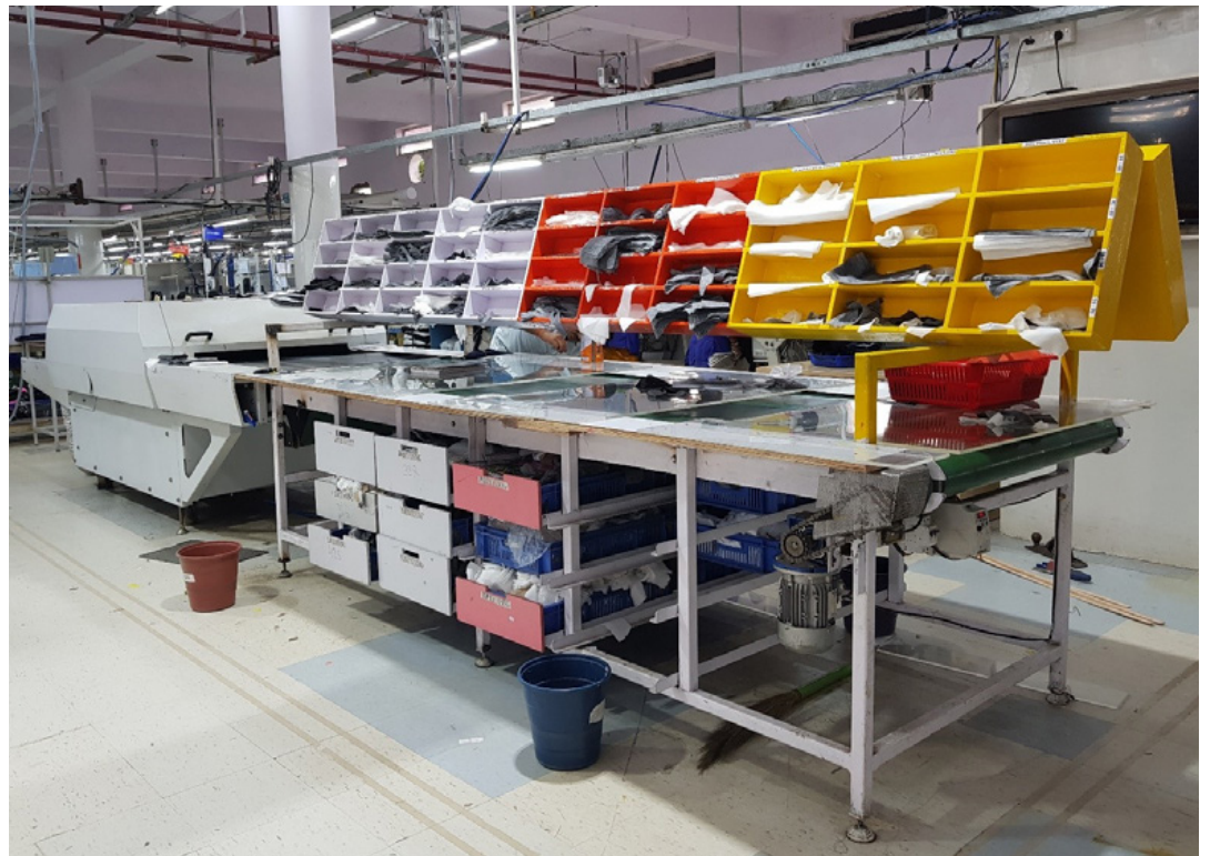
Fig: Fusing Machine Rack (After)
